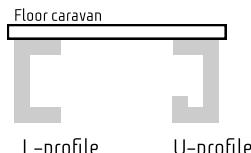
The chassis frames of caravans and trailers are classified into L- and U-profiles. They require different, additional fastening sets, depending on the vehicle and the installation conditions. These fastening sets are optionally available. Check the installation dimensions of your easydriver in Fig. 7.1.
